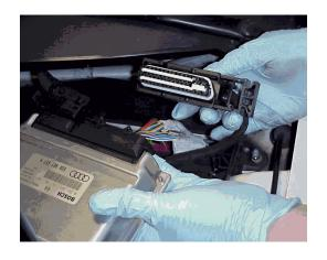
Attach electrical plugs to the ECM ensuring that the plugs are fully seated and release mechanisms are pushed all the way in. Snap sprung bracket back into place on top of ECM. Check that ECM is properly positioned in case.
