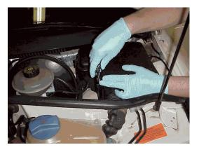
Loosen and remove the five 8mm screws attaching the Engine Control Module top cover to the case assembly. This is located in the rearmost section of the engine bay on the driver's side of the car.
